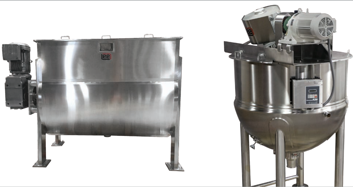
Compared to horizontal blenders (left) kettles with inclined agitation (right) offer major advantages in certain food processing applications.
